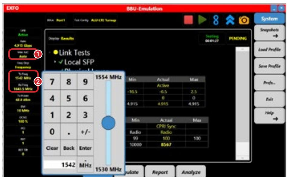
Figure 58. BBU emulation Tx frequency
