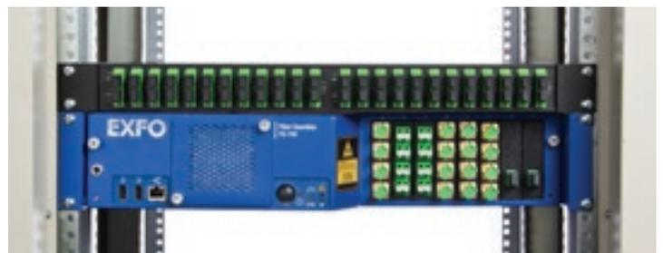
Figure 80. Configuration with 24 ports based on 12-f MPO and test access module kit (TAMK) that houses 24 WDMs, all occupying a 3U space
