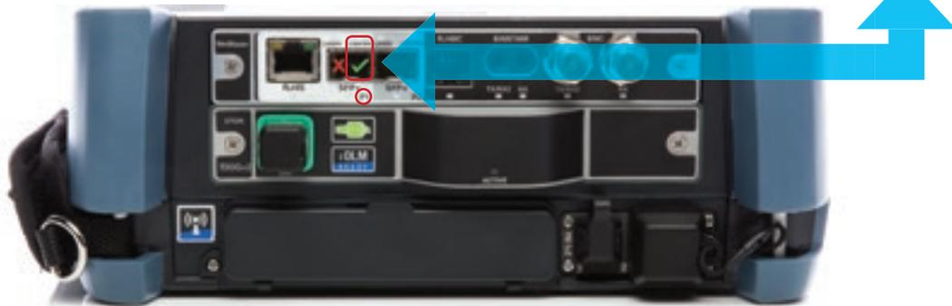
Figure 62. FTB-700G V2 Series and splitter (TAP) connections
