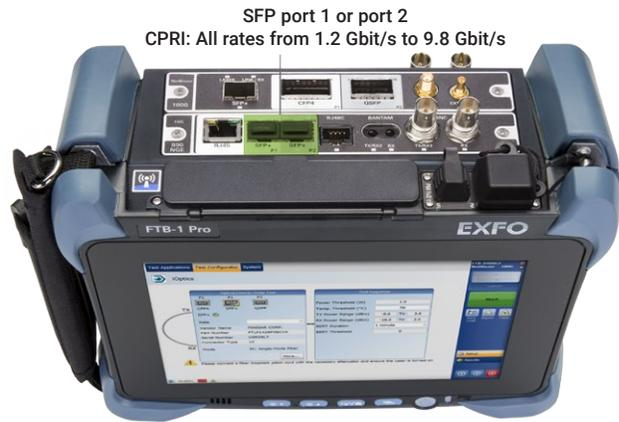
Figure 21. CPRI interfaces on the FTB-890NGE 100G module
