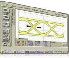
Figure 2. Example of an eye diagram at one of the outputs of the pB100A4
