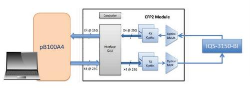
Figure 1. Typical setup for CFP2 testing
