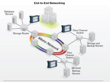
Thanks to end-to-end network testing capabilities, EXFO's Power Blazer enables fast deployment and configuration of Fibre Channel networks. Communication between the transport network, interconnection devices and end nodes can be validated with features such as BER testing, latency measurement, buffer-to-buffer credit estimation and port login capabilities.
