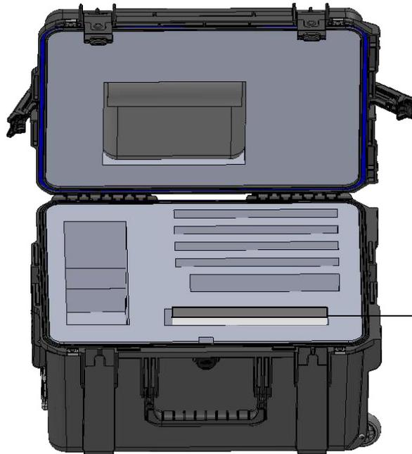
Place the FTB-5230S or FTB-5240S module in this location, with the input port and handle towards the left.
