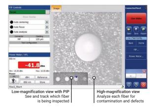
ConnectorMax2 also offers the smoothest MPO and MTP connector analysis process thanks to its unique PIP multifiber view, which is paired with the automated centering and focusing functions of the FIP-430/435. This leaves your hands free to control the *X* and *Y* scanning tool, enabling you to sequentially run the pass/fail analysis on each fiber of the connector in order to obtain a global status as per the standards.
