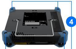
Using a flat screwdriver, turn the screws clockwise until they are tightened.
