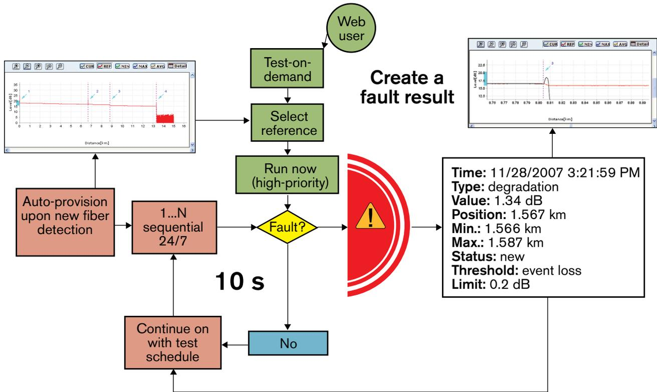
Monitoring and testing on demand functional diagram
