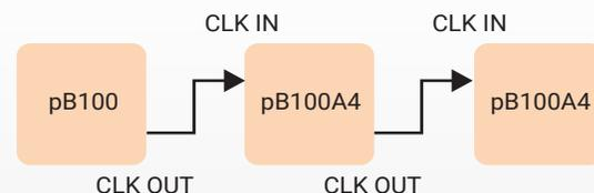
Figure 4. 3 pB100A4 connected to support 12 channel BERT
