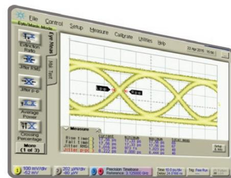
Figure 2. Example of an eye diagram at one of the outputs of the pB100A4
