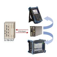
Power Blazer modules support G.709 testing in either the FTB-200 or FTB-500.
