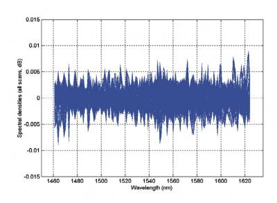
Impressive spectral density stability of the FLS-2200 broadband source (compilation of 30 scans, one per minute).
