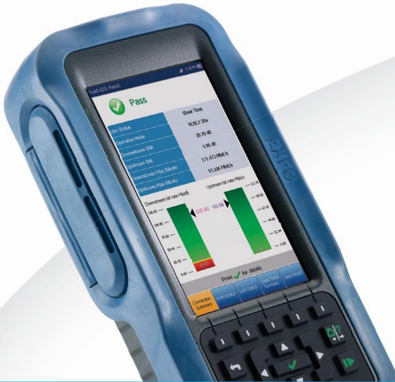
Fast, easy-to-use and cost-effective solution for installing FTx services over DSL.
