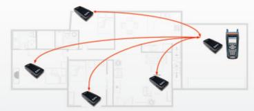
Prequalification of a coaxial environment for HPNA deployment.
