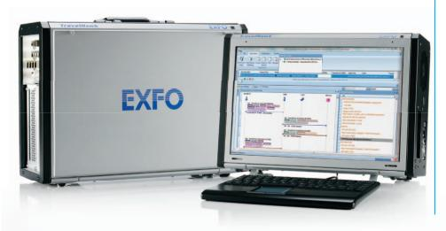
Troubleshooting a mobile network sometimes means leaving the comfort of the office and going on-site to investigate the problem. This requires an analyzer to be portable, without sacrificing functionality. The TravelHawk can be easily carried and stowed in the overhead compartment of an airplane. By avoiding the logistical problems of carrying cumbersome equipment to a site, test engineers can get to the field quickly to fix the problem.
