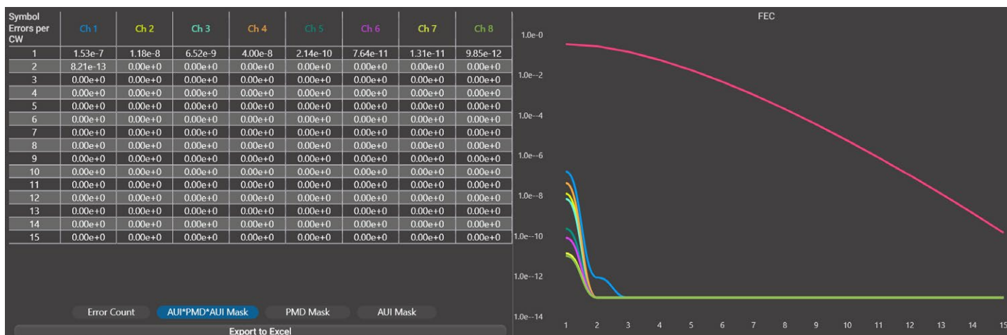
FEC channel distribution and BLER mask testing
