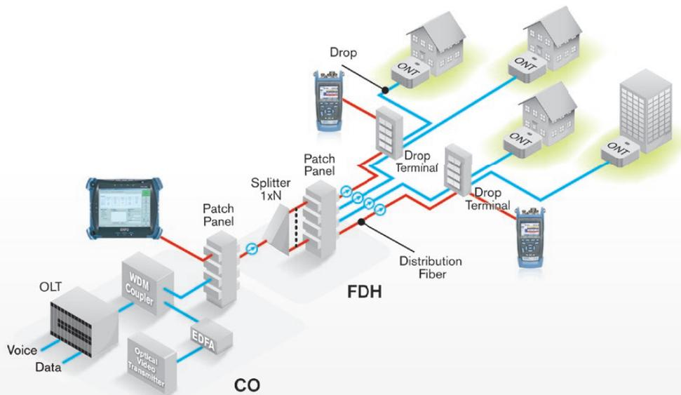
The FOT-930 allows for automated, bidirectional loss and ORL testing of passive optical networks (PONs) at 1310 nm, 1490 nm and 1550 nm, the three wavelengths recommended for PONs by ITU-T (G.983.3).
