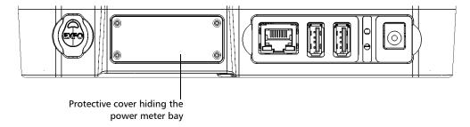
**6.** Using a screwdriver, remove the four screws of the protective cover.
