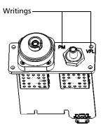
**9.** Carefully align the power meter with the corresponding bay.
