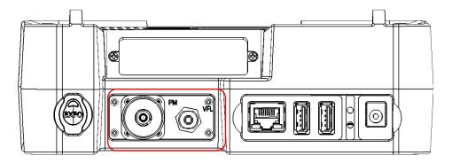
**Note:** If you have a protective cover for the power meter bay, keep the screws close at hand. You will need them to secure the protective cover in place later.
