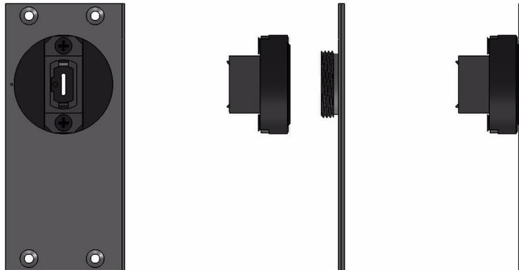
Below you can see the new FOA model and an old faceplate. Since the thread in the FOA is longer than the one on the plate, the connection is done fully, as you can see from the side and front views.
