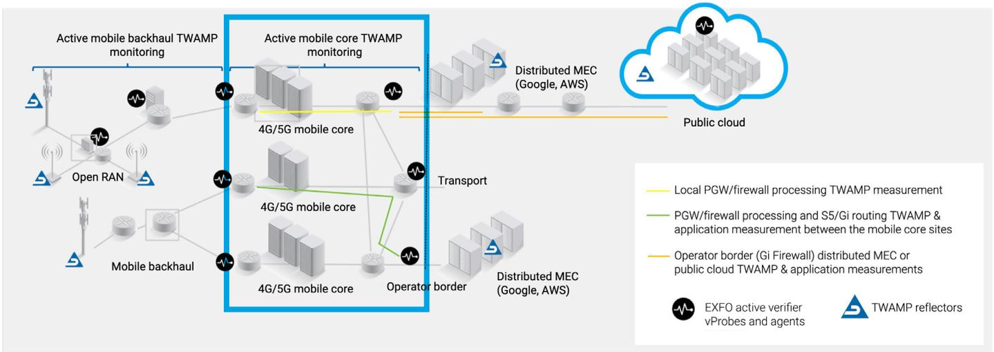
EXFO's active monitoring addresses mesh mobile core performance by injecting test traffic into an active GTP tunnel.
