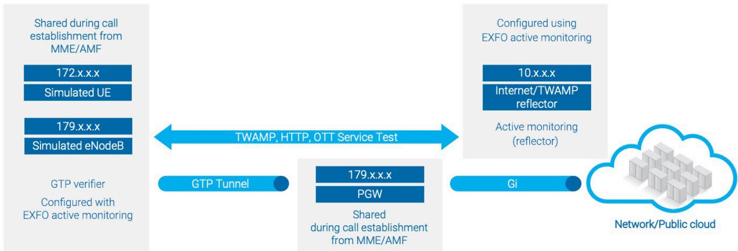
The tested service segment is the same as real customers are using through the APN configuration. The figure describes the simulation procedure and parameter exchange.
