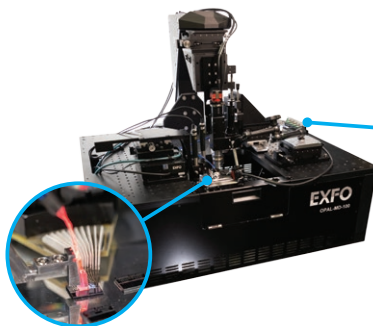
Figure 4. EXFO’s platform for multi-die testing comprising the OPAL-MD test station, EXFO Pilot software and EXFO test and measurement instruments for optical characterization of PIC. Third-party instruments can be added and controlled by EXFO Pilot.
