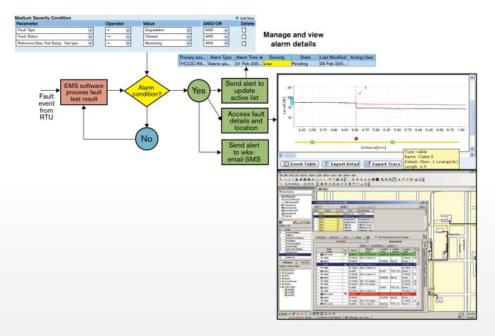
Alarm management and fault location on a linear and network map view
