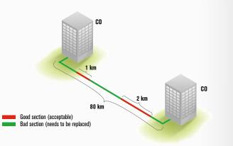
Distributed PMD analysis breaks down the measurement results effectively pinpointing the high-contributing sections of the link.
