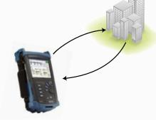
Using a single-ended instrument-a CD and PMD test tool that can characterize a section between two sites without having instruments at both ends-means that many sections can be characterized in a few minutes instead of a few hours from a single location. As a result, an entire network can be characterized greatly reduces truck rolls and OPEX, while increasing speed to deliver new services and reducing time-to-cash.
