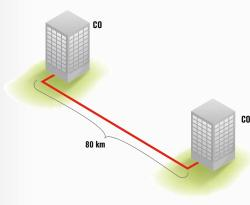
Traditional PMD measurement techniques provide a total link PMD value but do not locate which spans are causing the link to fail the test.
