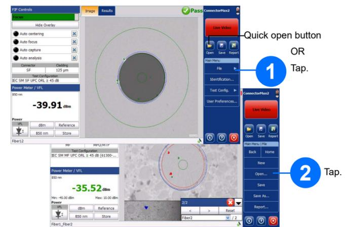
The FIP-400B Fiber Inspection Probe is a portable video microscope used to inspect fiber-optic terminations. Using ConnectorMax2, the dedicated software, you can view the fiber directly, or capture and analyze the results.
