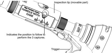
The icons on screen indicate when you can change the position of the inspection tip and the status LED as well. When the LED is blue and stops flashing, you can perform a capture.
