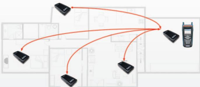
*Prequalification of a coaxial environment for HPNA deployment.*
