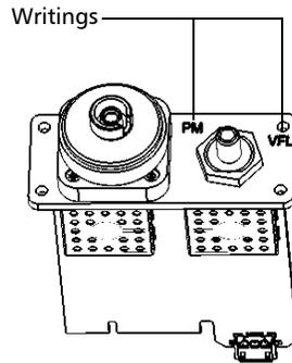
9. Carefully align the power meter with the corresponding bay.
