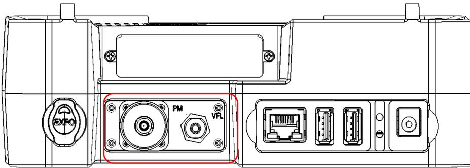
**Note:** If you have a protective cover for the power meter bay, keep the screws close at hand. You will need them to secure the protective cover in place later.
