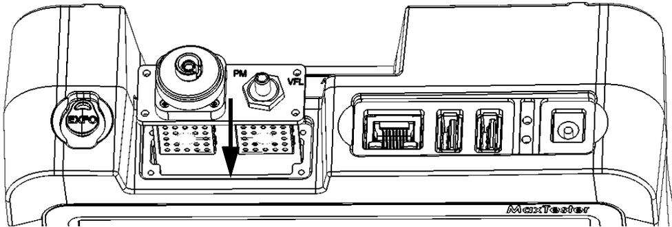
10. Gently slide the power meter into the bay until its faceplate is flush with the edge of the bay.
