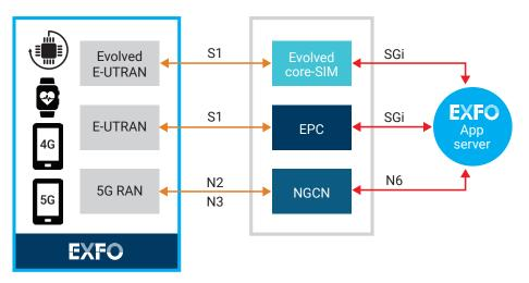
Figure 1. 5G core end-to-end testing
