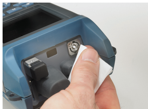
Figure 14: Cleaning the ferrule in the connector port.
