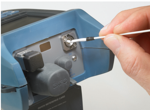
Figure 10a: Cleaning the detector port(s) using cleaning tips.
