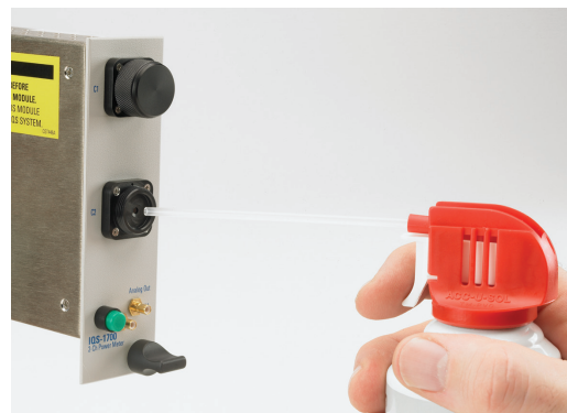
Figure 10b: Cleaning the detector port(s) using compressed air.
