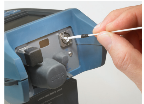
Figure 7: Cleaning bulkhead connectors.
