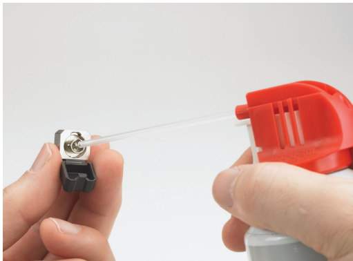
Figure 13: Drying the EUI with compressed air.
