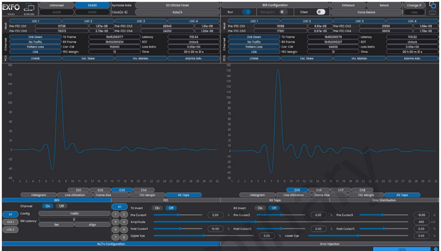
Figure 3. Detect ISI and far-end reflection.
