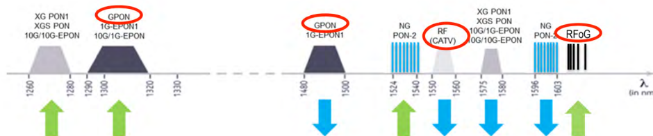
Figure 2. The different wavelengths that travel through the optical cable.
