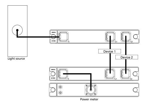
**2.** Measure the DUTs with the power meter.
