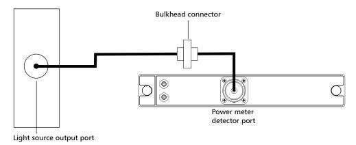
**2.** Store the power reading obtained as a reference value in the power meter.
