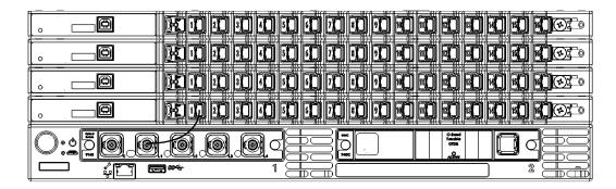
**Note:** Since the RTUe-9120 switch is equipped with unpinned MPO ports (two rows of eight fibers each), you will need a patchcord with a pinned MPO connector.
