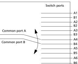
1 x N Duplex Optical Switch Principle
