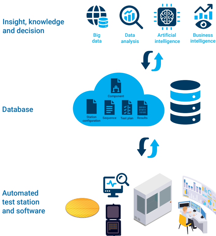
Figure 6. OPAL test stations and EXFO Pilot software automates PIC testing with powerful, scalable features, utilizing multiple applications linked to a collaborative database for advanced data analysis and AI.
