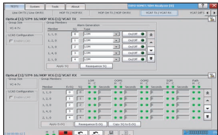
Figure 3. The 81x0 Next-Generation SONET/SDH module provides real-time GFP, VCAT and LCAS alarm and error analysis.
