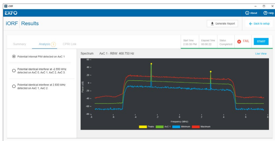
Figure 3. iORF results analysis indicating the source of interference and PIM, and their details.
