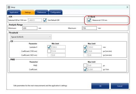
**5.** For the **Analysis Range**, enter minimum and maximum wavelength values. The analysis range is the value used to calculate the ITU grid and the maximum value for the acquisition. The analysis range can be different from the wavelength measurement range.
