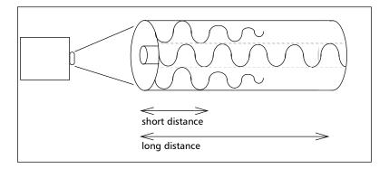
Due to the internal optics of the Variable Optical Attenuator (and the majority of attenuators), most of the cladding modes are filtered out. This means that, with the attenuator connected, the power meter will display a loss greater than the attenuation setting of the attenuator (cladding modes have been partially stripped).
