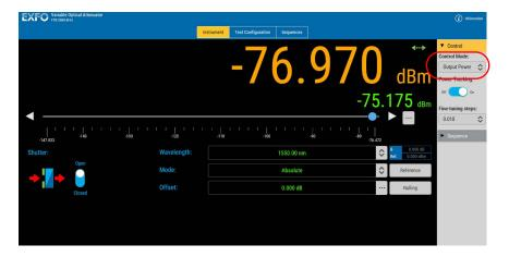
**3.** Switch the **Power Tracking** button to the ON position.
