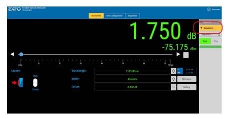
**Note:** Once a sequence is started, all controls in the **Instrument** function tab are disabled to avoid accidental interruptions.
