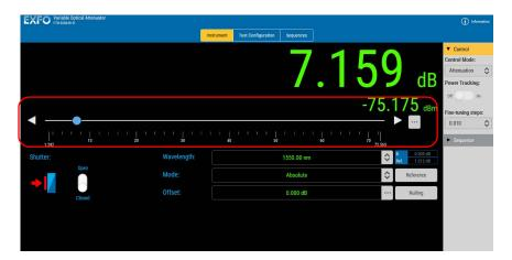
The offset value is not applied to a particular wavelength. It does not affect the filter attenuation. It can be used to compensate for the loss generated elsewhere in the system.
