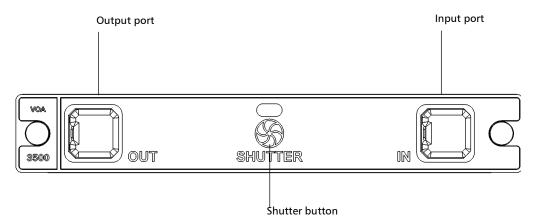
The module is configured for singlemode or multimode fibers and complies with optical return loss measurement (ORL) standards on transmission equipment.
