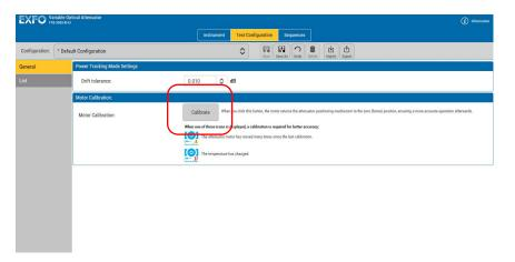
The attenuator mechanism is moved to the zero (home) position.
