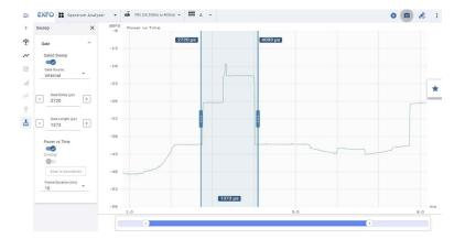
➤ Frame Duration (ms) allows selecting the X axis length of the Power vs Time graph: 10 ms (default) or 20 ms.
