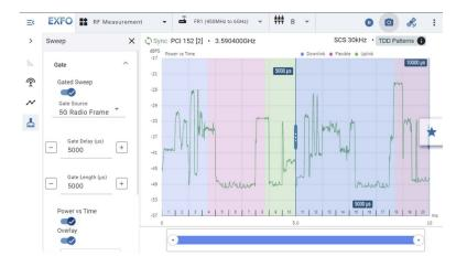
Using the color-coded graph, the gate delay/length can be configured to target a certain period of the radio frame (e.g. flexible slots when hunting interferers). This can be done by dragging the gate start and end on the graph, or by using the **Snap to Boundaries** mode. First, tap the **Snap to Boundaries** button and then:
