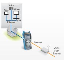
AXS-200/650 in Ethernet Through Mode (Ethernet Monitoring)
