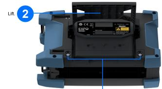
Turn the screws counterclockwise until the compartment door is loose.
