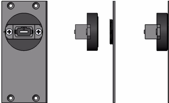
Below you can see the old FOA used on a new plate. The thread of the FOA is not deep enough and the connection is not complete. The FOA is not aligned properly when you look at it from the front.
