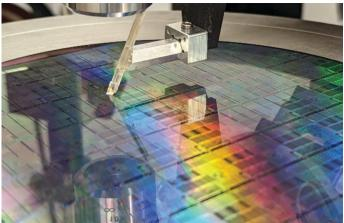
EXFO's OPAL automated test stations -Trench edge coupling
