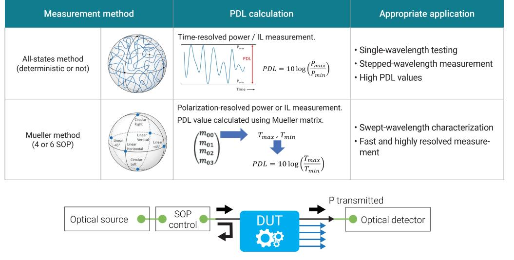
PDL measurement configuration
