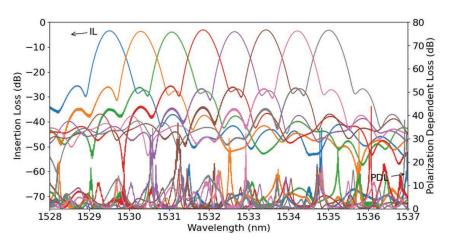
Multiport spectral response and isolation PDL of an AWG measured with a CTP10 platform
