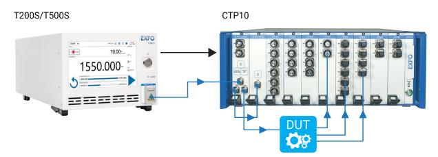
Typical IL/RL spectral characterization setup using a T200S/T500S with CTP10
