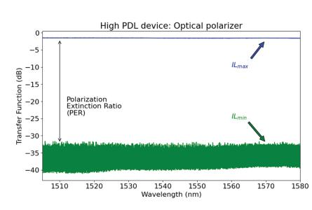
Maximum/Minimum IL of an optical polarizer using the CTP10 with external high-speed polarization controller
