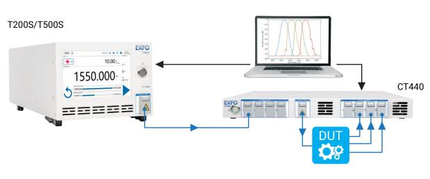
Typical IL spectral characterization setup using a T200S/T500S with CT440
