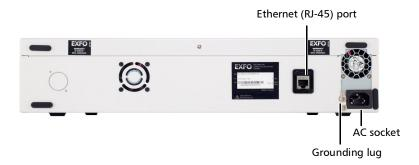
**Note:** For compliance to EMC requirements in industrial locations, a ferrite (Würth Elektronik P/N 74271131 or equivalent) must be placed on the Ethernet cable, near the Ethernet port on your instrument.
