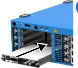
Insert the protruding edges of the module into the grooves and push all the way to the back. the way to the back.
